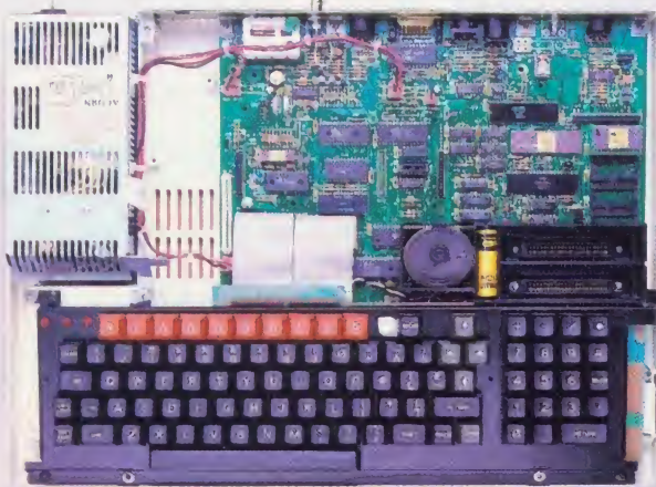
Master 128 with lid off: note break key guard and RAM battery by cartridge slots
